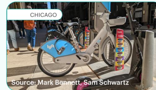
**Docking stations:** Docking stations include docks for the exclusive use of the shared micromobility system. Although docking stations are most commonly used for station-based bike share, some e-scooter share systems also include docking stations. In Chicago, Divvy Bikes modified docking stations to accommodate both bikes and e-scooters.
